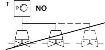
3 wires actuators **CANNOT** be connected in parallel to a single room thermostat / control unit.
