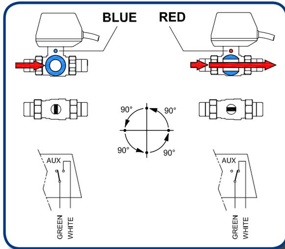
Utilisable fluids: water or liquids compatible with PTFE and EPDM. Before installing the valve be sure that no solid residues, like welding or threading residues, remain in the hydraulic circuit.
