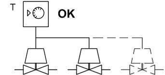
2 wires actuators **CAN** be connected in parallel to a single room thermostat / control unit.
